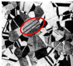
Micrograph of twinning in phosphor bronze
