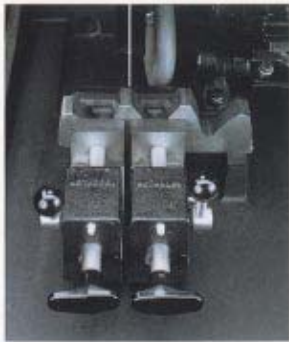
Cam activated vises (left hand vise standard) grip samples securely during sectioning.
