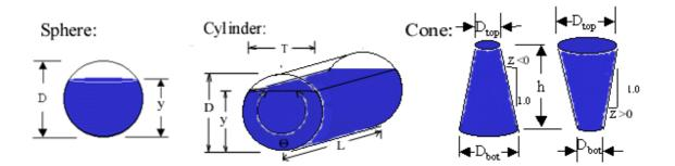
$$\begin{split} &\text{Sphere} \ : \ V = \frac{\pi}{3}y^2 \left(1.5\,D - y\right) \\ &\text{Cylinder} \ : \ V = \frac{L\,D^2}{8} \left(\theta - \sin(\theta)\right) \qquad T = 2\sqrt{y(D-y)} = D\sin\left(\frac{\theta}{2}\right) \\ &\text{Cone} \ : \ V = \frac{\pi\,h}{12} (D_{bot}^2 + D_{bot}D_{top} + D_{top}^2) \quad z = \frac{1}{2h} (D_{top} - D_{bot}) \end{split}$$
